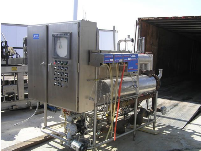
Figure 2 CIP System Control Panel and Chemical Boxes Reference Image
