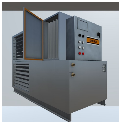
Figure 3 Glycol Cooling System (Unity View)
