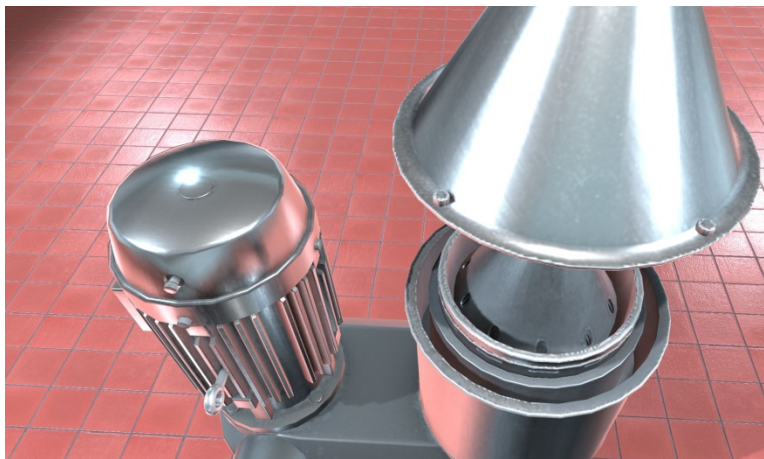
Figure 7 Separator and Separator Plate - Interior View (Unity)
